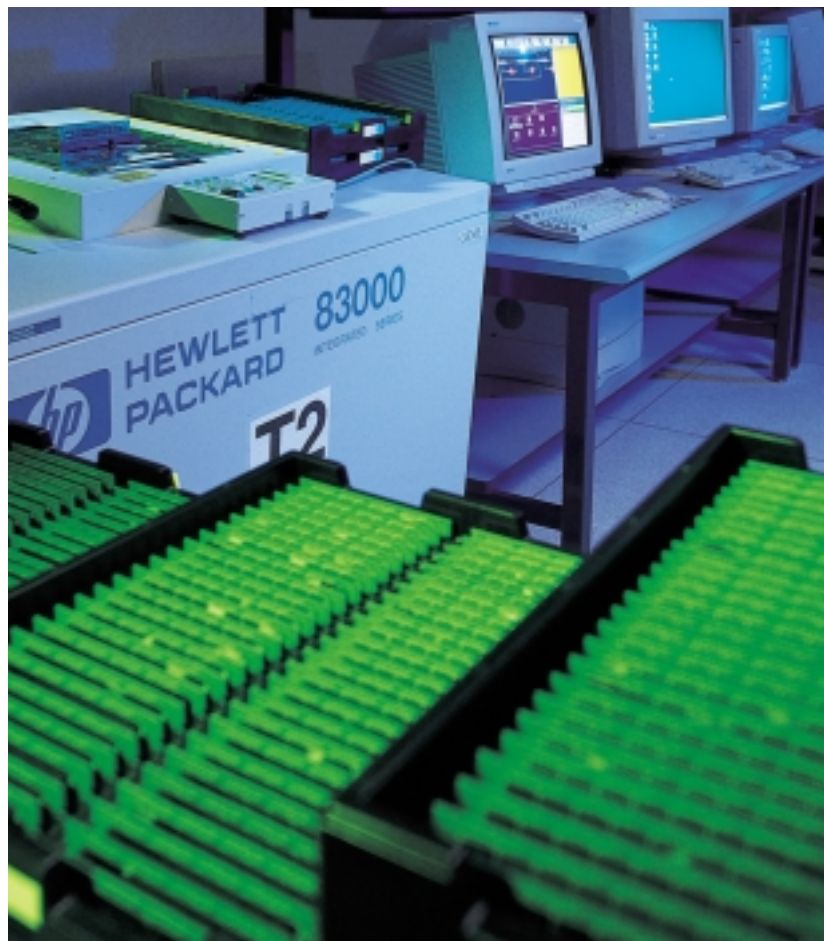
CUTTING-EDGE AGILENT 83000 TESTERS CERTIFY KINGSTON MEMORY MODULES.
