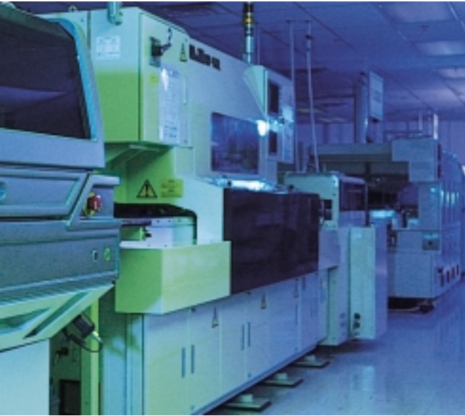
ONE OF THE SURFACE MOUNT TECHNOLOGY (SMT) LINES BUILDING SERVER MEMORY MODULES AT KINGSTON.
